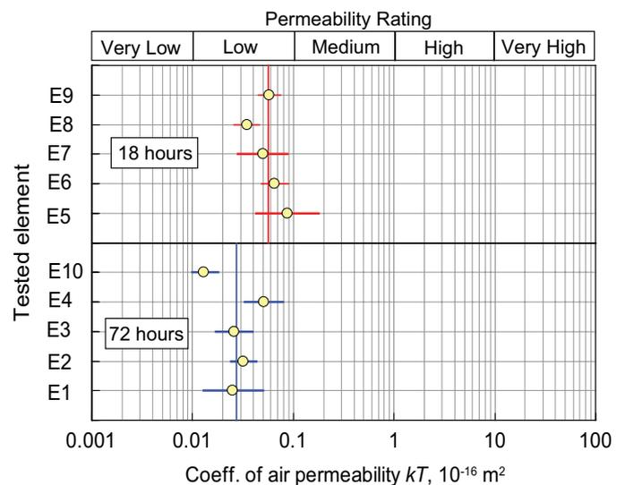
Fig. 7: Summary results for tested segments cured for 18 and 72 hours. Circles represent  $kT_{gm}$  values, and horizontal line segments represent  $\pm s_{LOG}$ . Vertical lines correspond to overall  $kT_{gm}$  of the data sets for the five elements in each curing category
