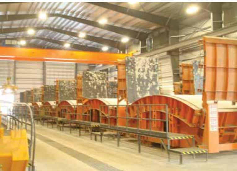
Fig. 1: A view of some of the 32 steel forms used for production of the tunnel lining segments
