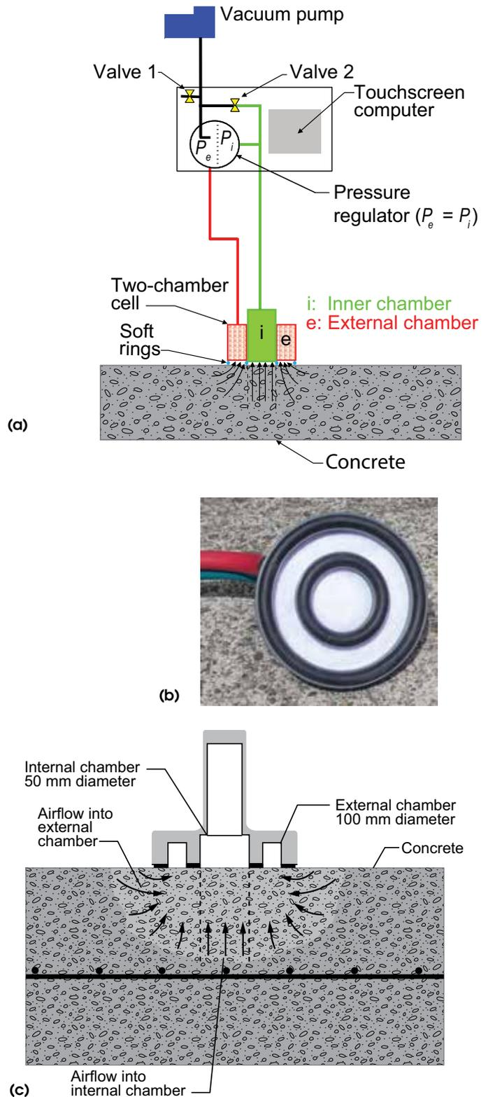
Fig. 4: A double-chamber vacuum cell was used to determine the coefficient of air permeability: (a) schematic of test setup; (b) detail of vacuum cell showing soft concentric rings and air hoses; and (c) schematic showing how the external chamber acts as guard ring ensuring unidirectional flow to the inner chamber
