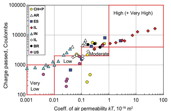
Fig. 8: Comparison of charge passed per ASTM C1202 and  $kT$  values per SIA 262/1-E,<sup>9</sup> from Reference 8. The data were taken from numerous sources. Permeability classes for the two test standards are also shown
