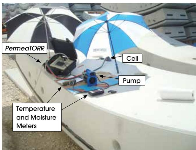
Fig. 5: During air permeability tests, the instrumentation was shielded from direct sunlight. As this image also shows, the formed surfaces of the segments were almost completely free of any “bugholes,” indicating a well-consolidated concrete
