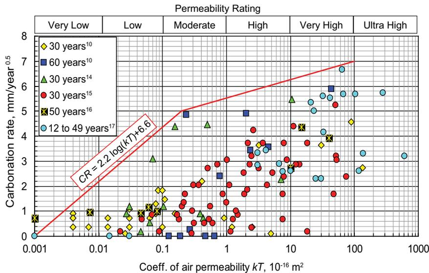
Fig. 9: Carbonation rate versus air permeability measured on old structures in Switzerland and Japan<sup>13-17</sup>
