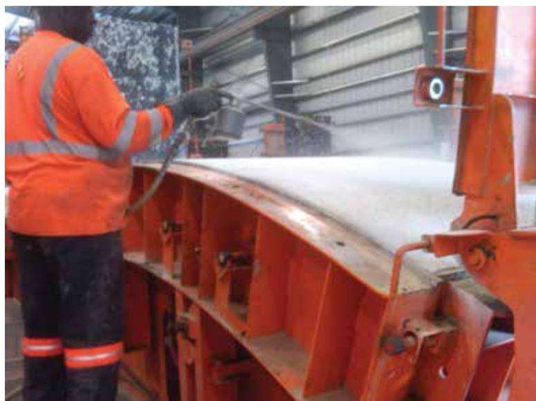
Fig. 3: The finished extrados of each segment was sprayed with curing compound
