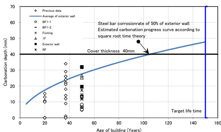
Figure 4: Carbonation progress of concrete by small core sampling test
