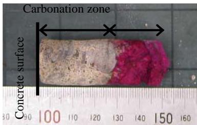
Photograph 3 : Carbonation of specimens
