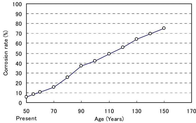
Figure 9: Progress of steel bar corrosion rate in north-side exterior wall
