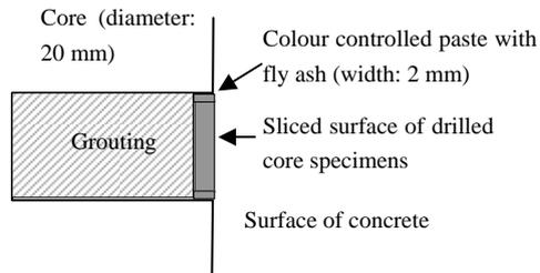
Figure 3 : Schematic description of repair of drilled hole
