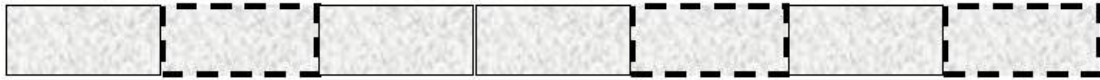
Fig. 1 – Example of the selection of Test Areas on 7 tunnel elements (60m 2 each), built at a rate of 1 per week; the areas marked with broken lines are the selected Test Areas
