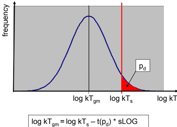
Fig. D-3: Normal distribution of logarithms of  $kT$  with a proportion  $p_d$  of “defectives” ( $kT > kT_s$ )
