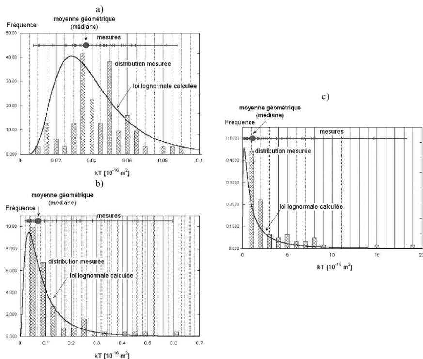
Fig. D-1: Distribution of Air-permeability test results from three jobsites with  $w/c$  ratios of a) 0.42, b) 0.52 and c) 0.73, Conciatori (2005)
