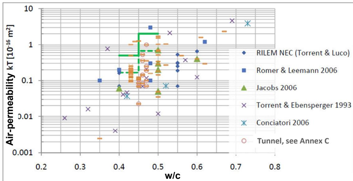
Fig. D-8: Proposed limiting values and geometric mean values from published research; orange symbols correspond to test results of concrete structures tested on site
