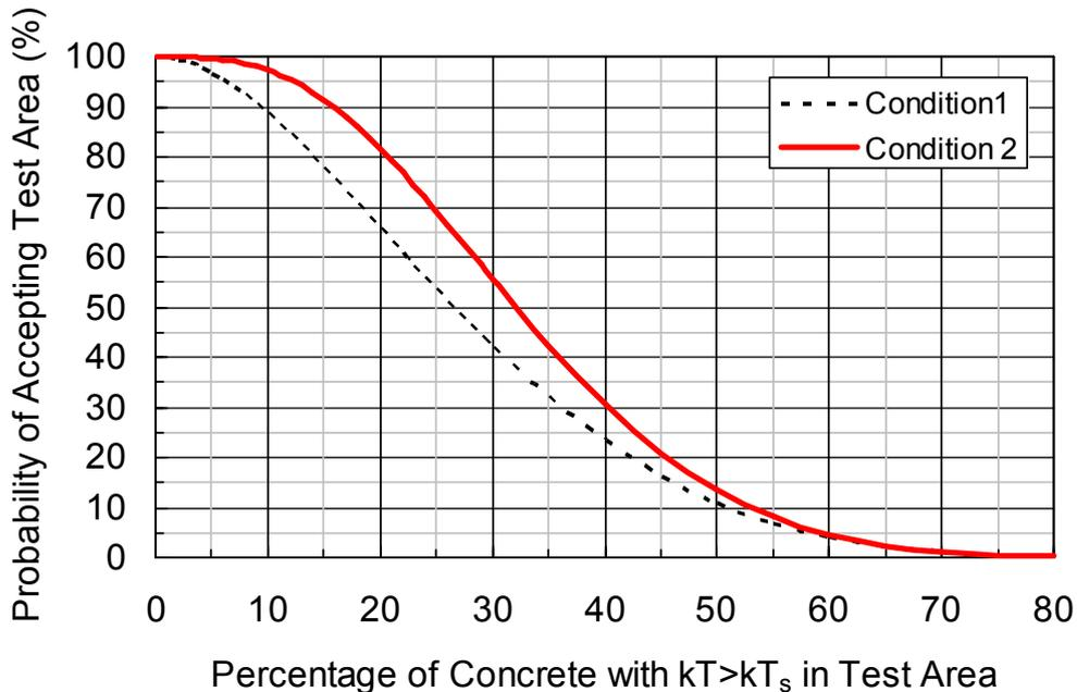
Fig. D-5: Probability of Acceptance Curve for the proposed Conformity Criterion <sup>5</sup>
