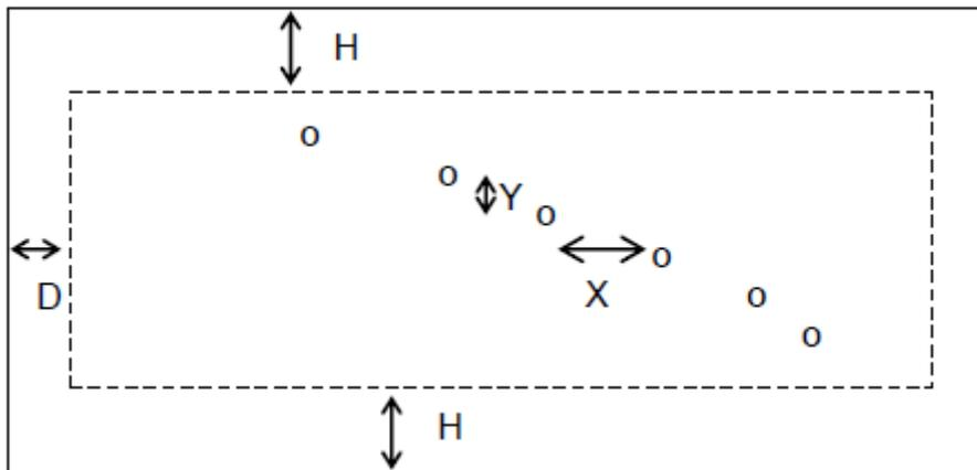
o: Measurement Point;  $H > 150$  mm,  $D > 50$  mm,  $X$  and  $Y > 200$  mm
