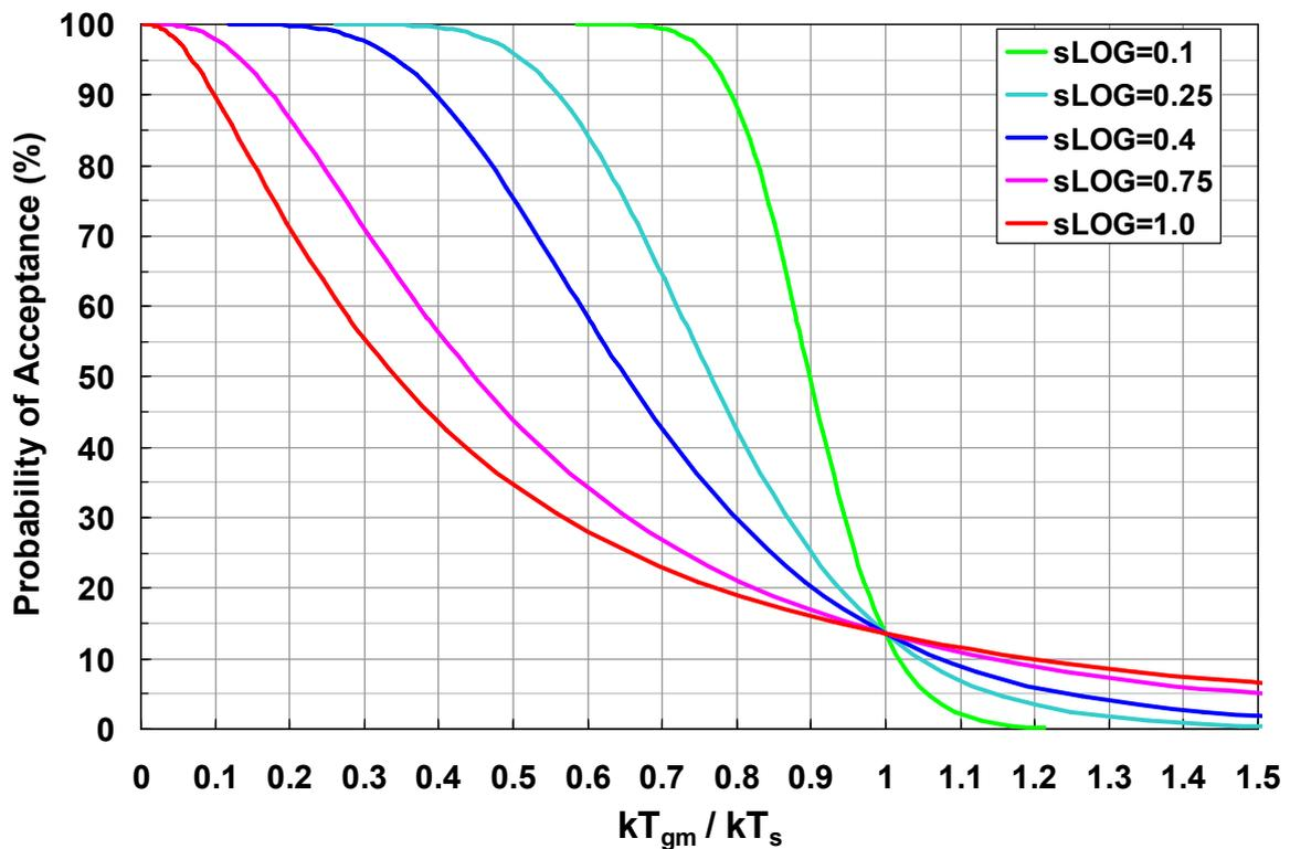
Fig. D-6: Probability of Acceptance as function of  $kT_{gm} / kT_s$  ratio and standard deviation sLOG
