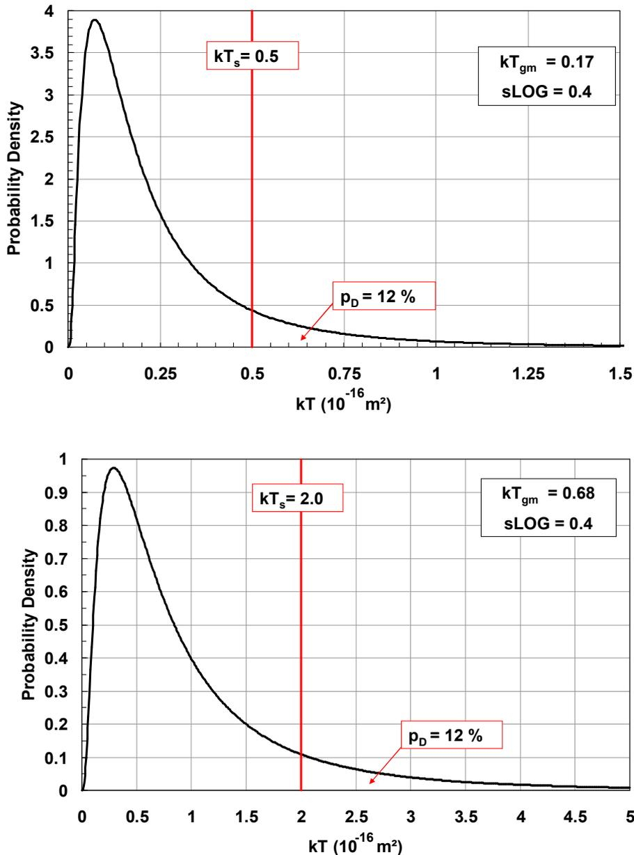
Fig. D-7: Probability Density distributions of  $kT$  for Probability of Acceptance 95% and  $sLOG = 0.40$ , for  $kT_s = 0.5 \cdot 10^{-16} \text{ m}^2$  (top) and  $2.0 \cdot 10^{-16} \text{ m}^2$  (bottom)
