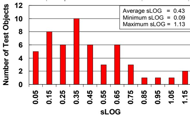
Fig. D-2: Standard deviation sLOG from 52 concrete elements, Jacobs (2006)
