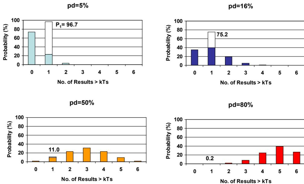
Fig. D-4: Binomial distribution for 6 tests for different proportions  $p_d$  of “defectives”
