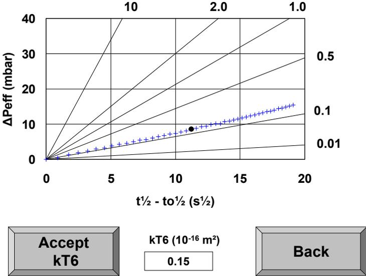
Fig. 6 – Display of *PT* instrument, with test results (+) and reference  $kT$  lines. The black dot is the value at  $t=360$  s ( $kT6 = 0.15 \cdot 10^{-16} \text{ m}^2$ ), which may be accepted by the user.
