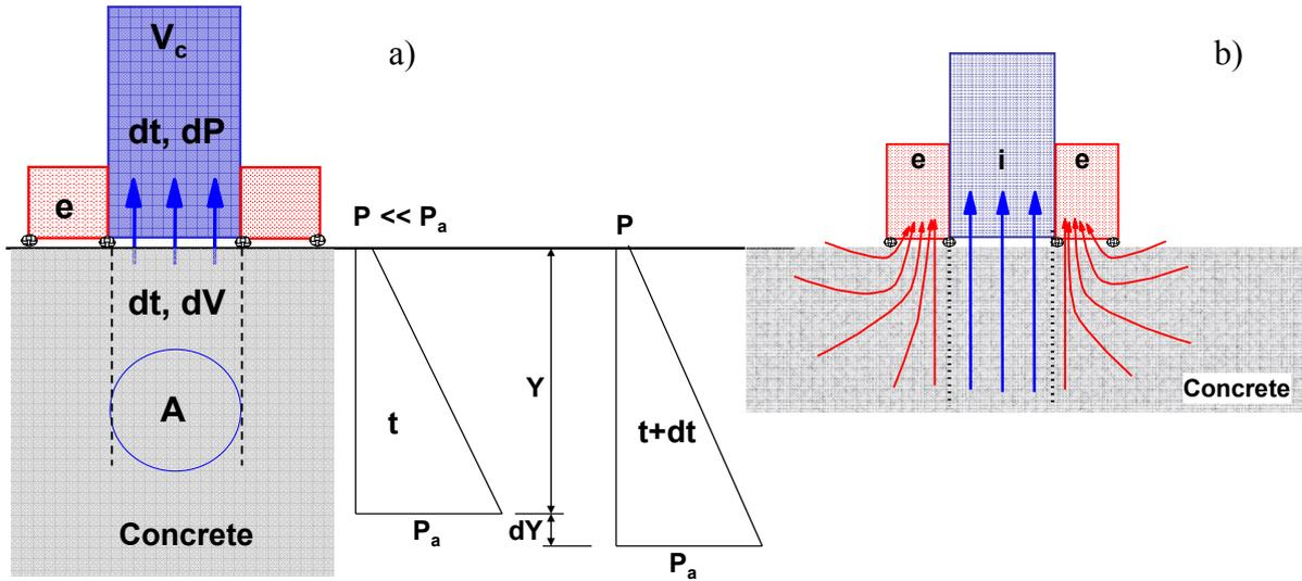
Fig. 3 – Main elements of the Model (a) and schematic air flow assumed (b)
