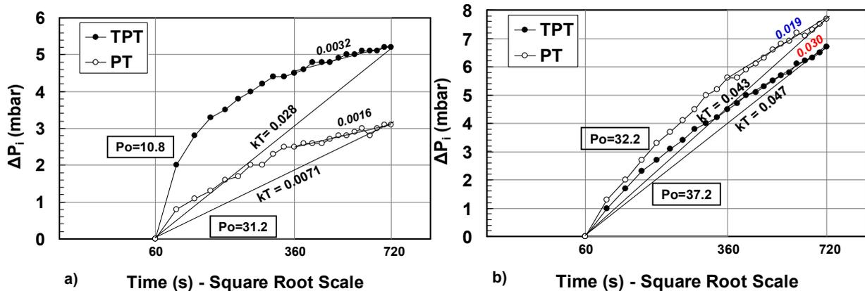
Fig. 4 -  $\Delta P_i - \sqrt{t}$  relations obtained with TPT and *PT* on two faces of a sample.
