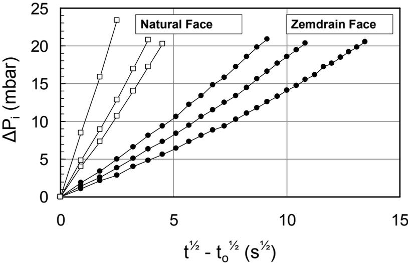
Fig. 7 -  $\Delta P_i - (\sqrt{t} - \sqrt{t_0})$  plot recorded on a panel one of whose faces was cast against a Zemdrain membrane.
