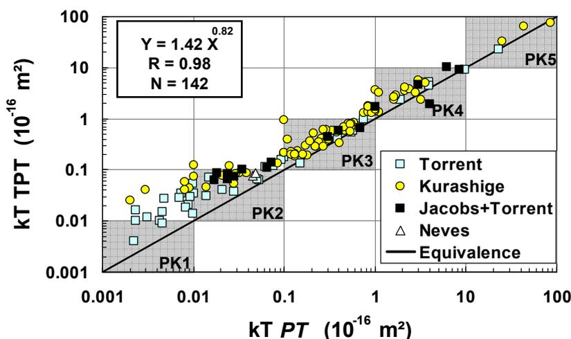
Fig. 5 – Correlation between the  $kT$  values obtained with the TPT and *PT* instruments by different researchers
